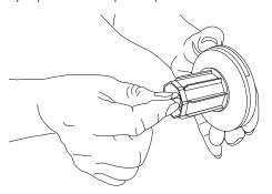
d) Open up the sprocket cage.
