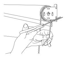
g) Replace the connector. Make sure the bottom of shade aligns with connector.
