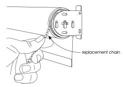
d) Using a small screwdriver, rotate the sprocket until the new chain comes out the back of the clutch.
