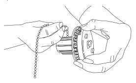
f) Place the new chain, making sure that the beads fit properly in the sprocket wheel.
