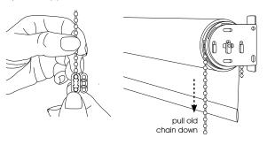
c) Place the new replacement chain on the sprocket. See drawing below.
