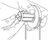
j) Push clutch back into the roller tube. Make sure the clutch key drives align with the roller tube drives.
