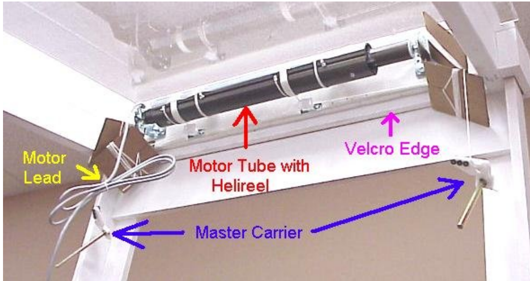
Figure 4 Motor Headrail Attached
