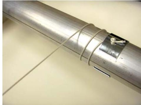
Figure 21 Return Cord Wrapped Over Tube
