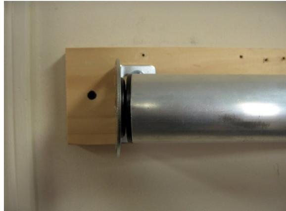
Figure 18 Motor Idler Collapsed in Bracket
