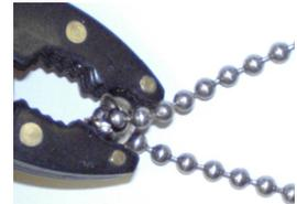
Figure 14 Crimp the Metal Stop
