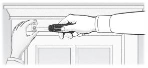
Ensure that the L-brackets are level and evenly spaced before attaching the shade.
