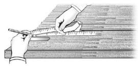
Use one of the Yankee brackets to mark the mounting locations. Align the bracket at each marked location, placing the bottom of the horizontal piece of the Yankee bracket at the same level as the top of the headrail. Mark the bracket mounting hole locations on the wall, at least two per bracket, and make sure that the brackets are level with each other.
