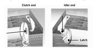
Motorized Lifting System-First place the idler end in its bracket on the headrail. Then, drop the motor end into its bracket, making sure the limit switches are easily accessible. Insert the cotter pin in the motor end, and bend the tabs so it cannot slip out. Adjust the limit switches as needed (instructions included separately).
