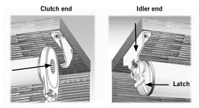
**Motorized Lifting System**—First place the idler end in its bracket on the headrail. Then, drop the motor end into its bracket, making sure the limit switches are easily accessible. Insert the cotter pin in the motor end.
