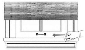
To raise the shade, pull the cord straight down until the shade is raised to the desired position. To lock the shade, pull the cord past the outside edge of the shade and release. Wrap excess cord around cleat.
