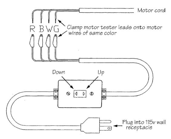
Use the motor tester to test and adjust the shade motor. To use the motor tester:
