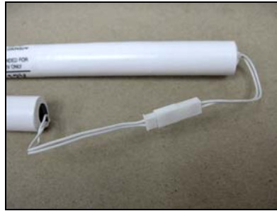
Figure 5 Battery wands connected
