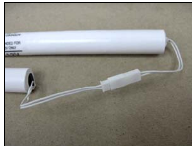
Figure 35 Battery Packs Connected
