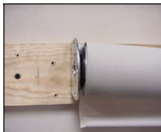
Figure 18 Idler Pin Collapsed in Bracket
