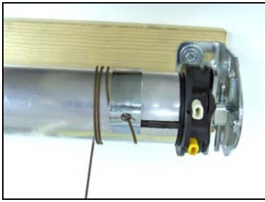
Figure 18 Cord Wrapped on Motor Tube
