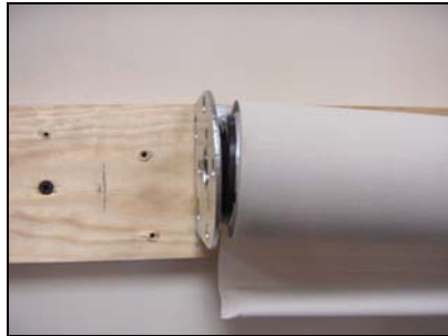
Figure 11 Idler Pin Collapsed in Bracket
