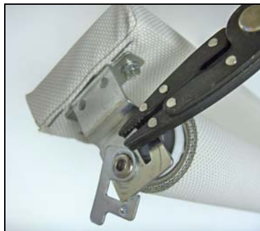
Figure 6 Placing Spring Pin in Spring Roller Bracket
