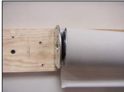
Figure 10 Idler Pin Collapsed in Bracket
