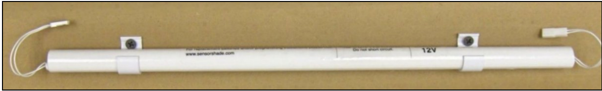
Figure 32 Battery Pack Attached To Brackets
