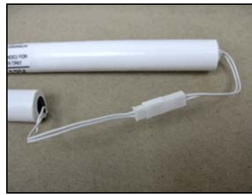
Figure 31 Battery Packs Connected
