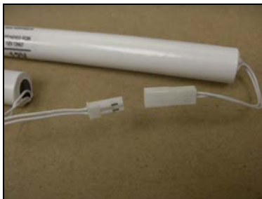
Figure 30 Battery Pack Connectors
