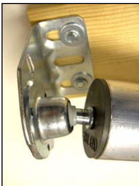
Figure 22 Motor Idler Going into Bracket
