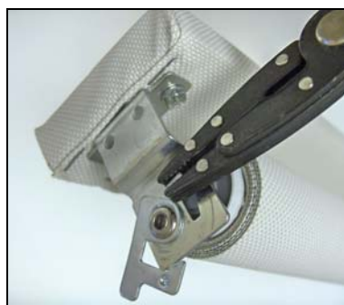
Figure 5 Placing Spring Pin in Spring Roller Bracket
