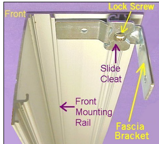
Figure 4 Fascia on Bracket (shade bracket removed for illustration)
